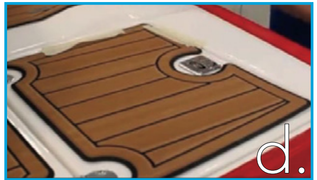
Tape one side down in exact location
