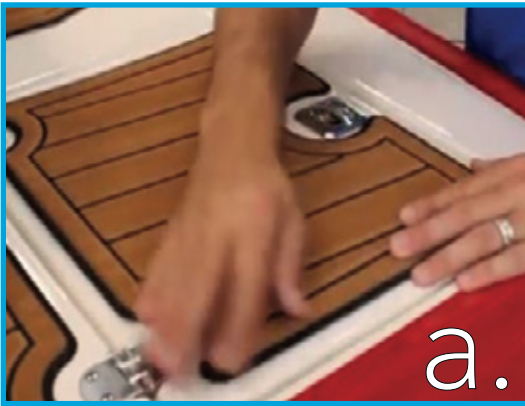
Verify fit and exact location
